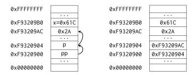
Let's assume that int\* p is located at 0xF9320904 and int x is located at 0xF93209B0. As we can observe:
