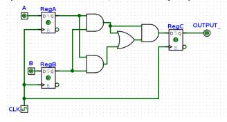
The maximum allowable hold time for RegC is how long it takes for RegC's input to change, so (clk-to-q of A or B) + shortest CL time = 4 + (5 + 5) = 14 ns.
