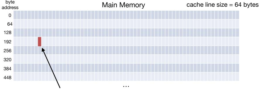
If we want to write to byte 199<sub>10</sub> and its not in the cache, we would bring in bytes 192<sub>10</sub>-255<sub>10</sub> into Berkeley EECS the cache and then update the byte
